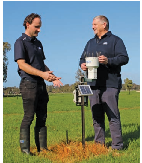
Summit Fertilizers Field Research Officer Sam Marsh (above left) shows Regional Sales Manager - Southern WA, Gary Lewis the CropX weather station and soil sensor installed at the Serpentine pasture trial. The availability of this exciting new technology will enable the collection of valuable site-specific data including temperature, rainfall and moisture held within the soil profile. The soil probe also measures soil electrical conductivity and can detect vertical movement of nutrients (such as nitrogen) down the soil profile after leaching events.
